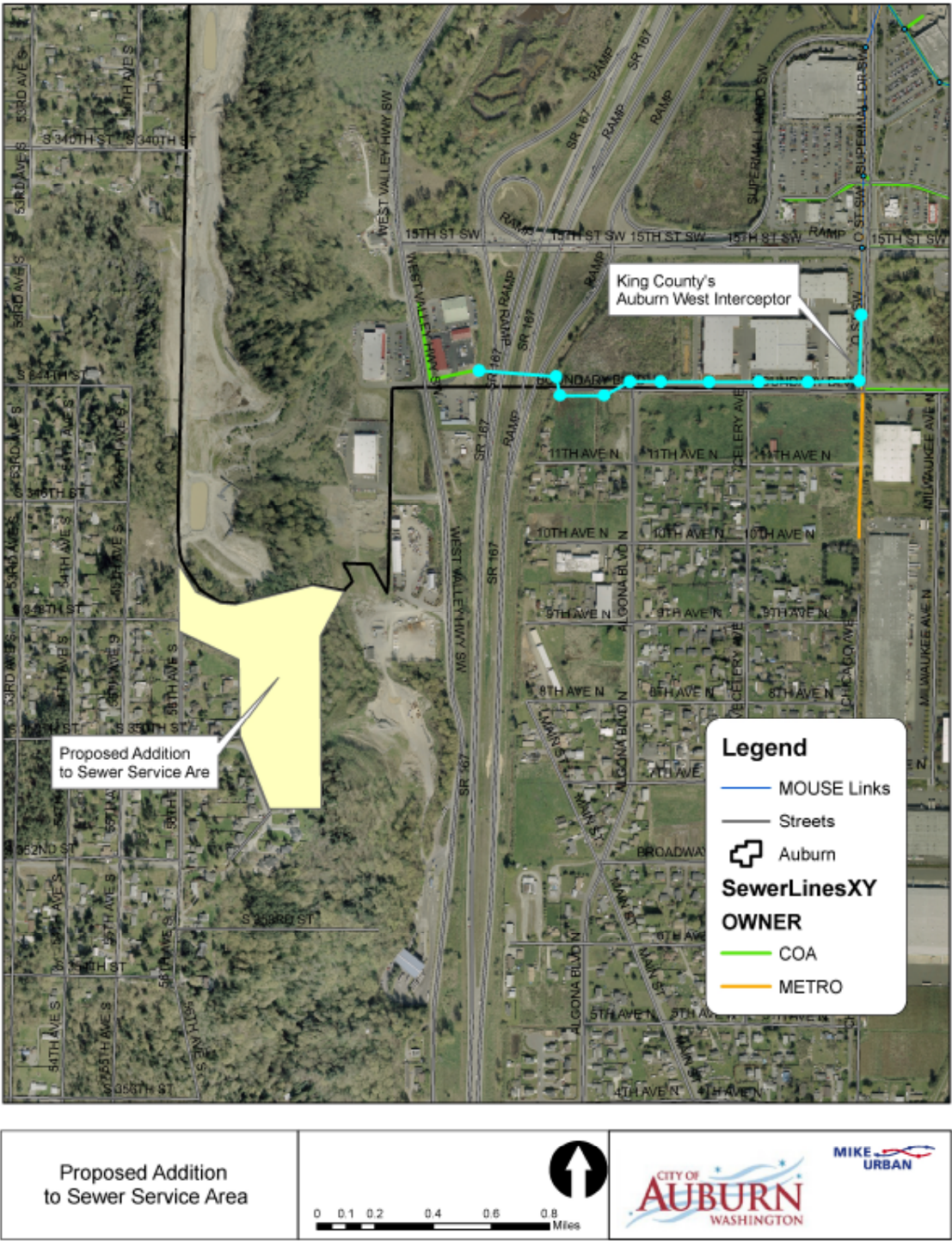
Figure 3-5. Proposed Jovita Annex area and downstream sewer pipes included in capacity analysis.
