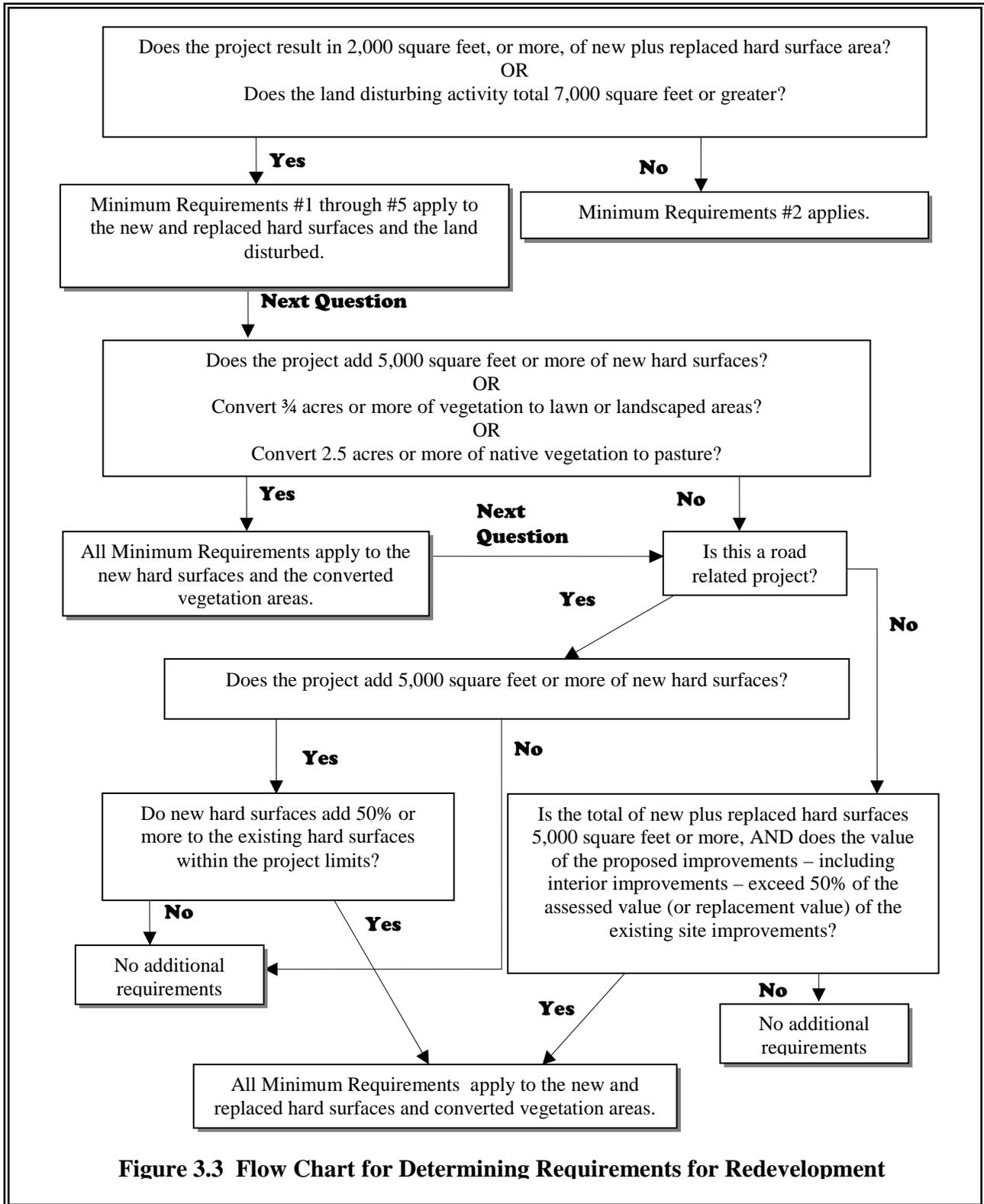
**Figure 3.3 Flow Chart for Determining Requirements for Redevelopment**
